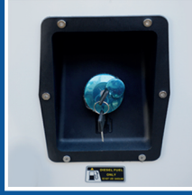
Diesel filling with key lock
