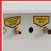
Oil and coolant drain
