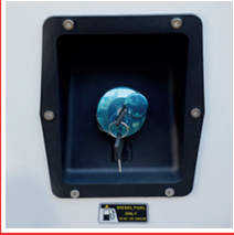
Fuel filling point with key lock
