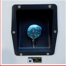
Fuel filling point with key lock
